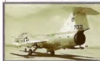
▲ Single engine The Starfighter was powered by a single J79 engine, the same one that powered the later F-4 Phantom in twin-engined configuration.
